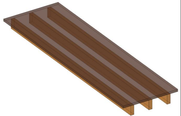
Figure 1-3: Open box with three webs and protruding flange
